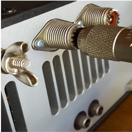
Coax Center Conductor Only—measure noise level
